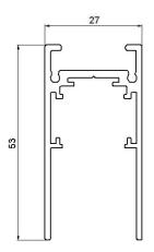
Dimensions: 4000 x 53 x 27 m Max voltage: 48 V, 10 A
